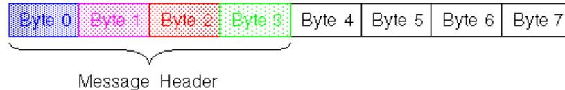
Figure 7.2-1. AGATE Data Bus Message Emphasizing the Header Structure
